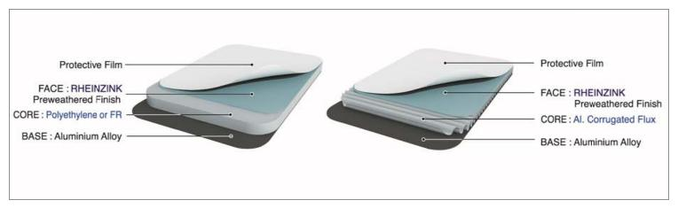
ZCM composite metal panels are adaptable to various installation methods including:
